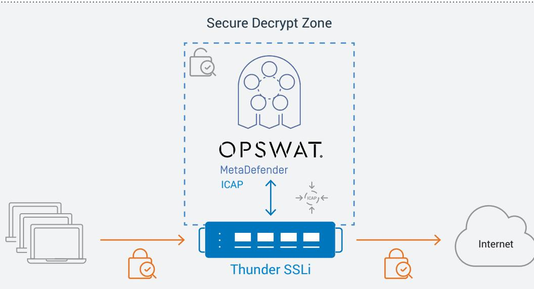
Figure 1: OPSWAT MetaDefender ICAP Server integration with Thunder SSLi
