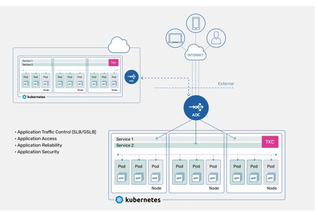
Figure 1: External access to Kubernetes applications in multi/hybrid cloud with A10 TKC and Thunder ADC
