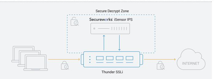
Figure 1: Thunder SSLi and iSensor IPS offer a collaborative solution that inspects bi-directional traffic inline, to mitigate malicious attacks hidden in encrypted traffic
