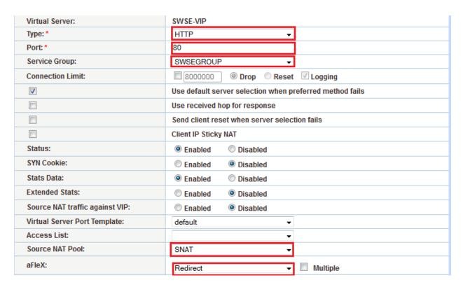
Figure 24: Source NAT and aFleX configuration
