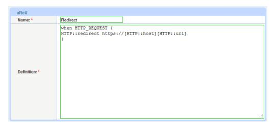
Figure 15: aFleX redirect configuration
