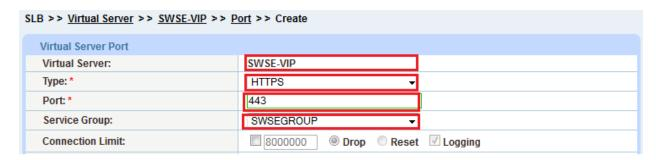
Figure 21: Virtual Server Port Configuration
