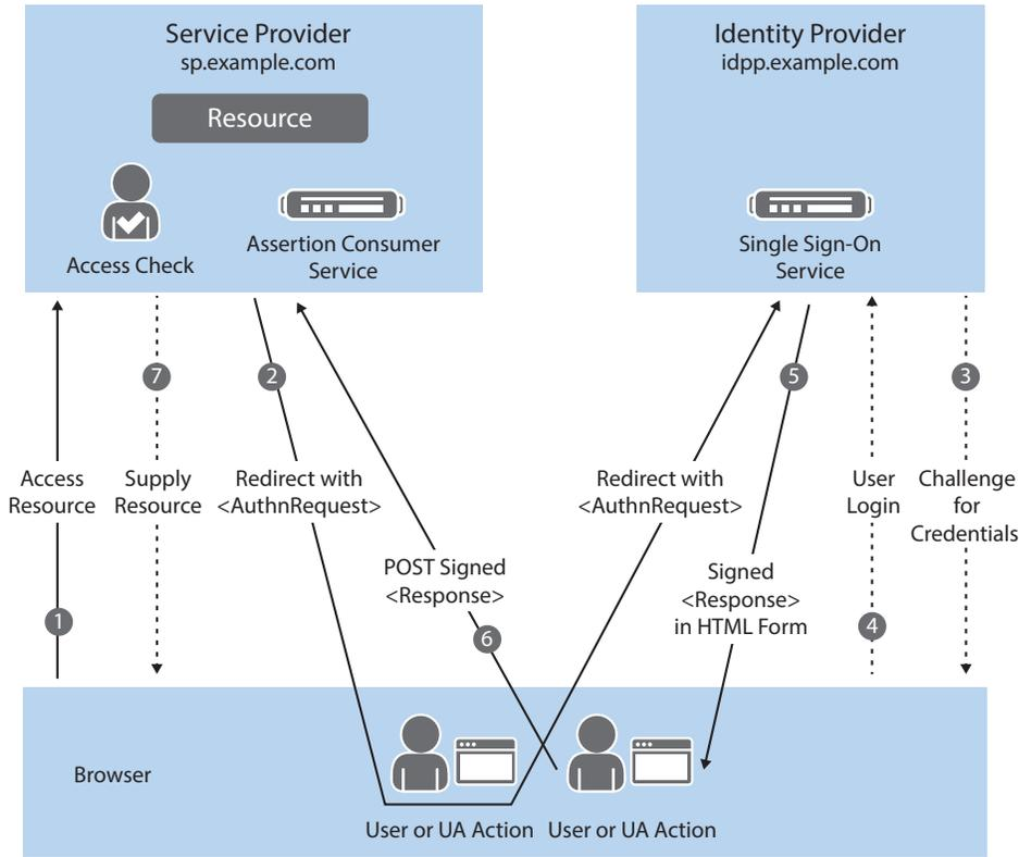
Figure 20. Frontend/service provider initiated
