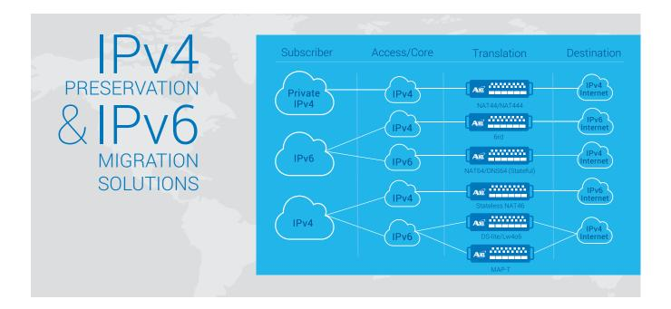
Each address and protocol translation technique provides a solution that allows a subscriber to transparently access content regardless of the protocol stack their device is using, the provider's access and core network support for IPv4/IPv6 and the destination server support. The available translation techniques support either tunneling or native protocol translation.
