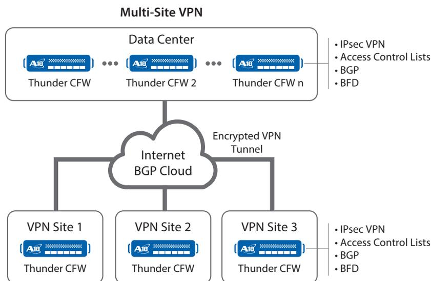
Figure 1: Thunder CFW can connect to multiple VPN sites over a BGP cloud
