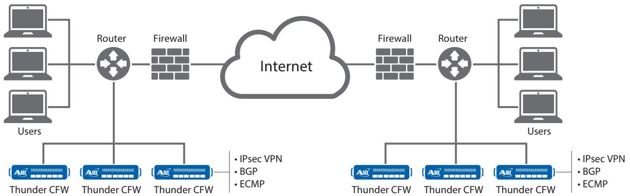
Figure 2: Users can forward traffic destined for the remote VPN site through the Thunder CFW appliance and send all other traffic directly to the Internet
