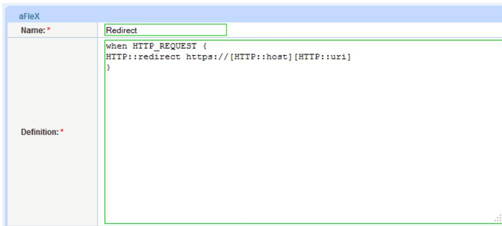
Figure 15: aFlex redirect configuration
