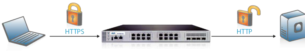
Figure 27: SSL Offload Overview
